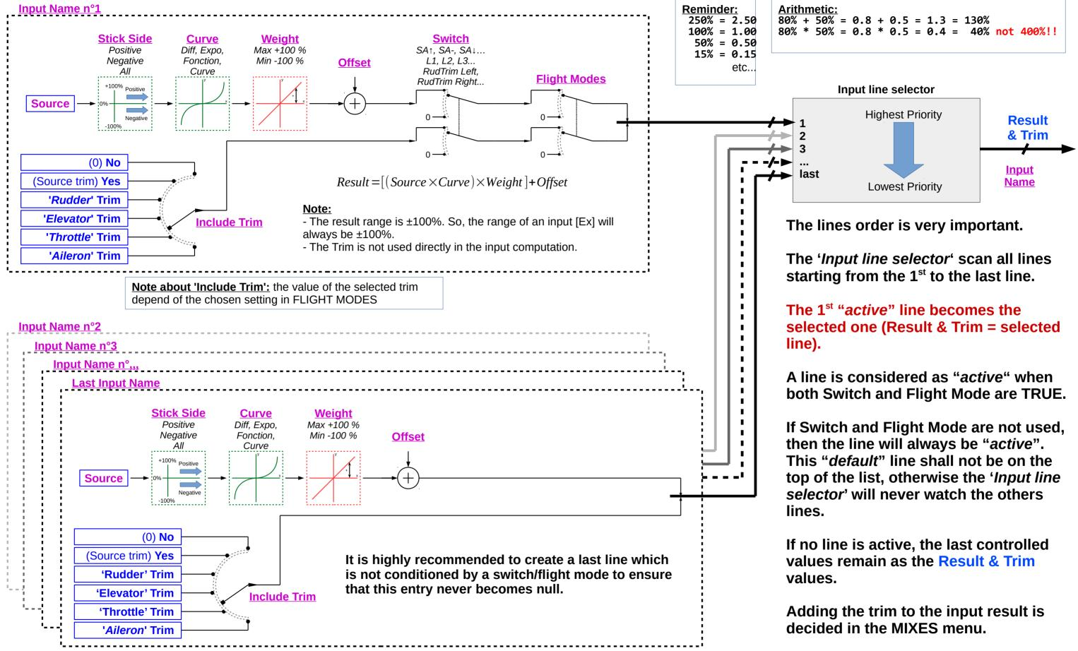
If the INPUT is used in the HELI or LOGICAL SWITCHES menu, then Result & Trim are added together
